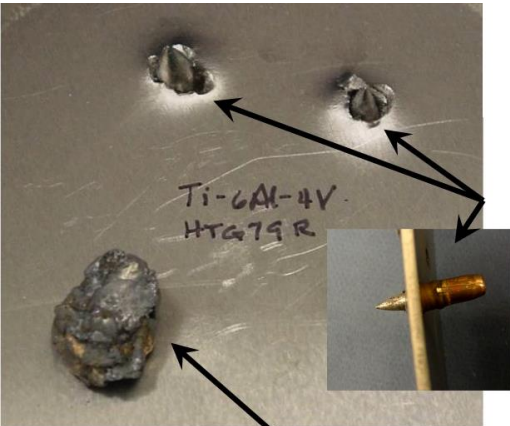
APM2 after impact with ceramic armor
